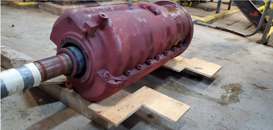
Figure 2: Volute from Unit 1 Boiler Feed Pump (Identical in East and West Pumps of Unit 1 and Unit 2)
